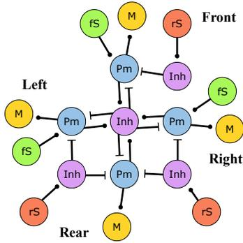
Fig. 2. The decision-making network implemented in Flyintel. “fS” stands for a foraging sensory neuron, “rS” stands for a risk-detecting sensory neuron, “M” stands for a motor neuron, “Pm” represents a premotor neuron and “Inh” is an inhibition neuron.
